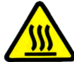
Figure 5 Warns user of heated hot surface hazard
